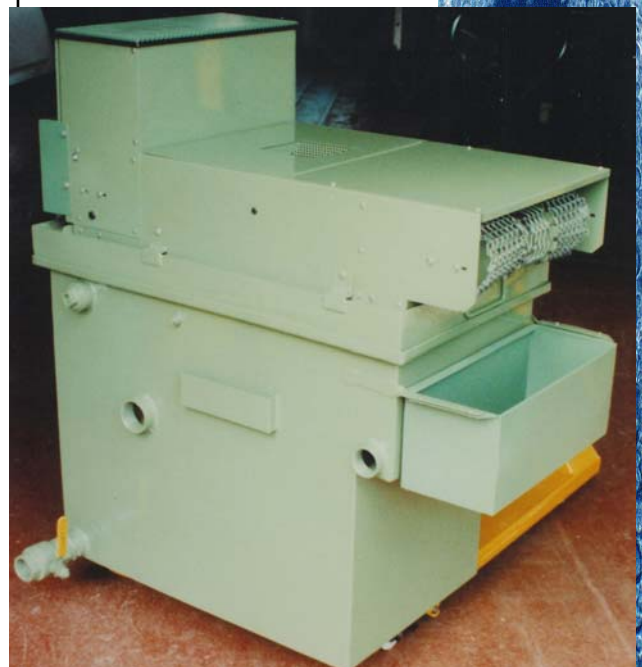
Filter unit hinge mounted on top of a Multipack tramp-oil separator
