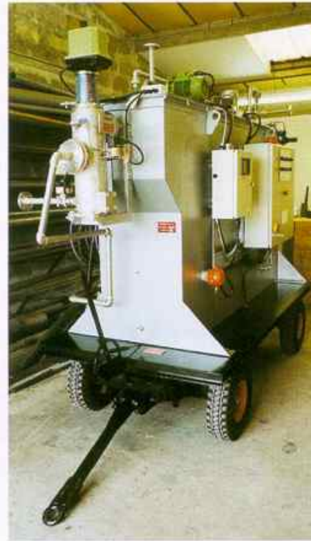
Mobile Stetpack TS6 separator with self-cleaning inlet strainer and oil-water monitor
